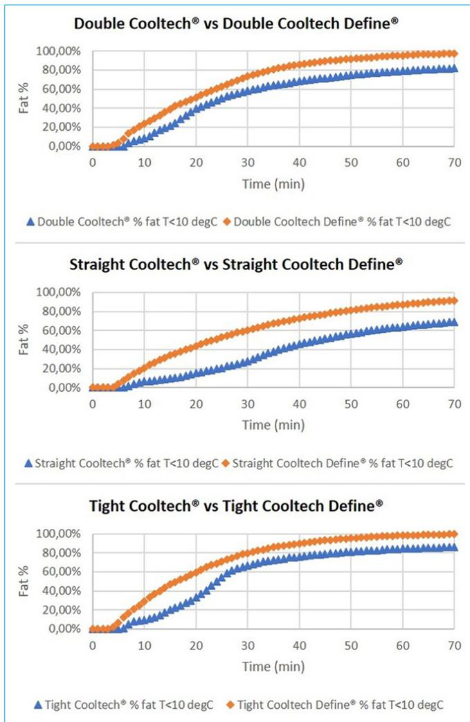
**Figure 12.** Fat % below 10 °C vs. time chart: Cooltech® vs. Cooltech Define®.
