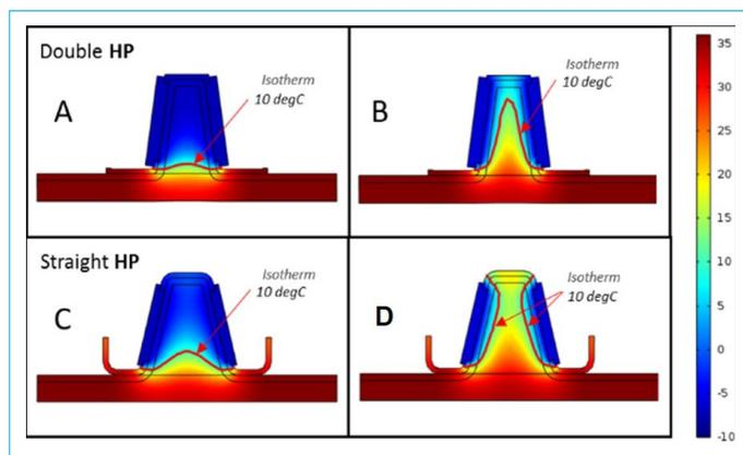
**Figure 15.** Cooltech® Double applicator without internal perfusion (A) and with 27% perfusion (B); Cooltech® Straight applicator without internal perfusion (C) and with 55% perfusion (D).
