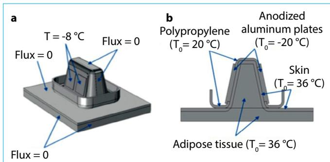
**Figure 5.** Boundary conditions (A) and initial conditions (B) used. Abbreviations: T, temperature, °C, degrees Celsius.
