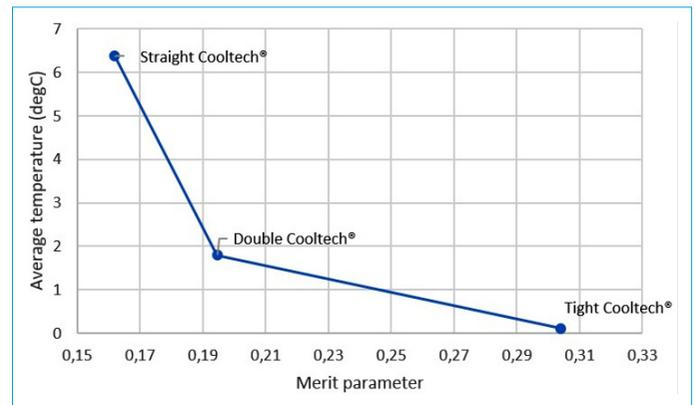
**Figure 7.** Fat average temperature at 70 minutes of treatment vs. the merit parameter for Cooltech® Straight, Double and Tight applicators.
