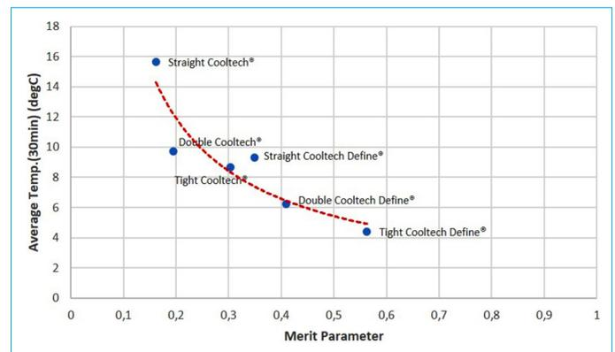
**Figure 8.** Fat average temperature at 30 min vs. the merit parameter for each Cooltech® and Cooltech Define® applicator. Abbreviations: Temp. temperature; min, minutes; degC, degree Celsius.
