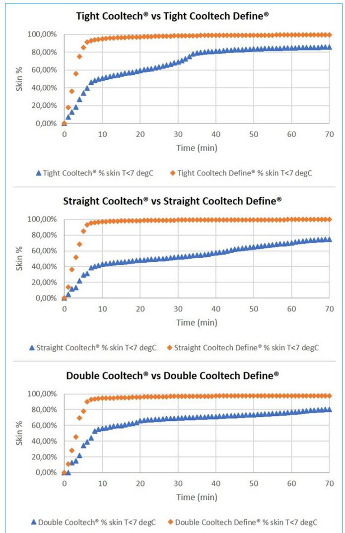
**Figure 13.** Skin % below 7 oC vs. time chart: Cooltech® vs. Cooltech Define®.
